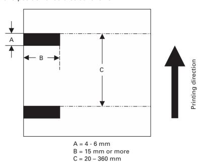
The distance from PE sensor and print head is approx. 7.5 mm.
